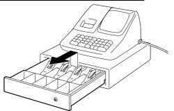
Pull out the drawer all the way until it hits the stopper. Then lift up the drawer and pull it again.
